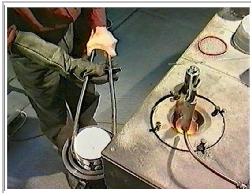
The flask needs to be seated squarely in it's cradle. The rubber o-ring on the bench top will be placed on top of the flask as a seal for the vacuum.
