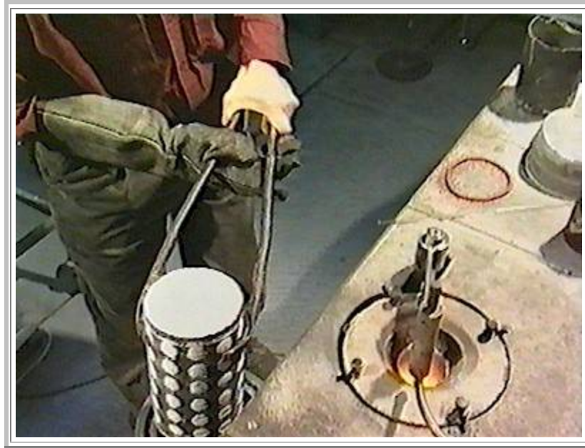
The flask is placed in the casting chamber.
